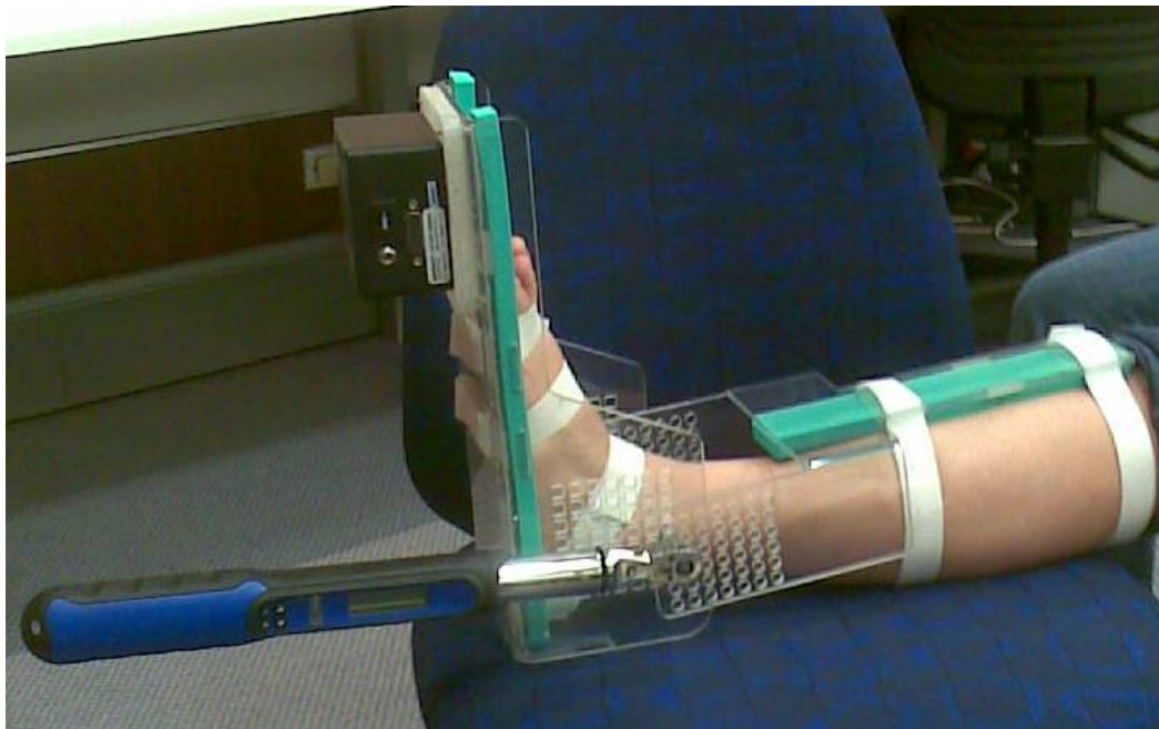
Figure 1: Charles device for measuring ankle dorsiflexion
