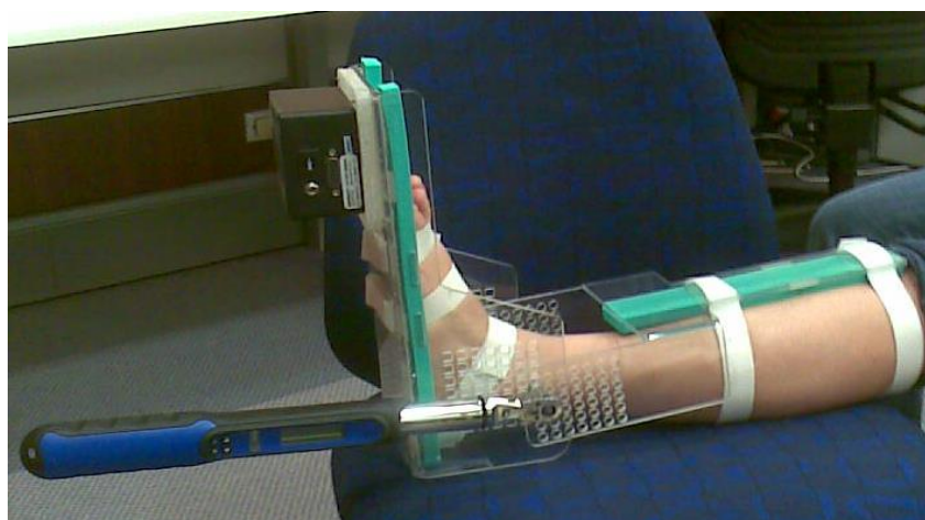
Figure 4: Charles Device to measure ankle dorsiflexion, Charles 2016 (24).
